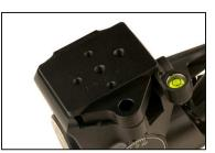
Place adapter plate at top of Manfrotto head.
