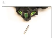
Remove Pin from safety mechanism and save it. You will need it later in step 6.
